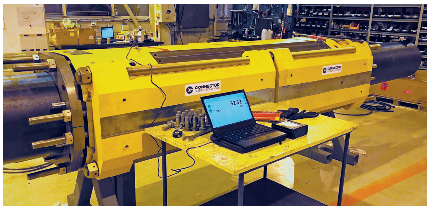
01 // Conductor clamp pressure testing
