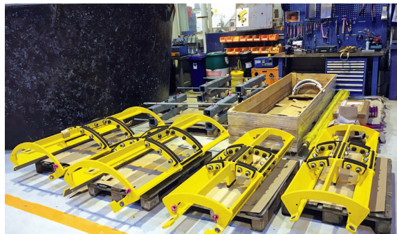
03 // Conductor centralizer fitted to clamp upon successful installation
