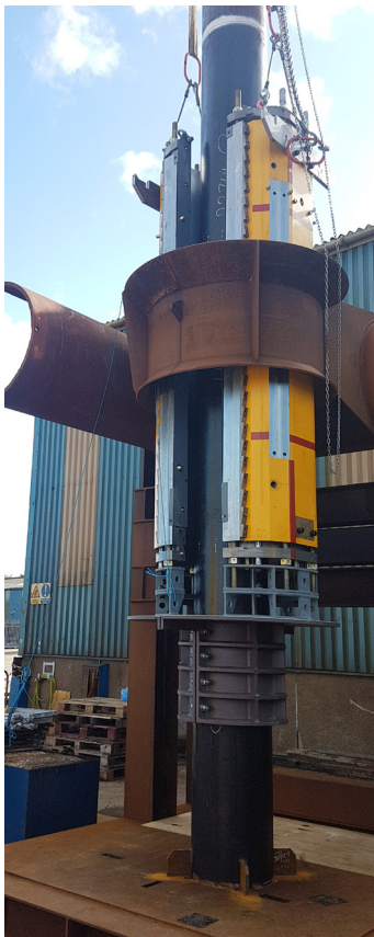
02 // Conductor clamp system integration test assembly
